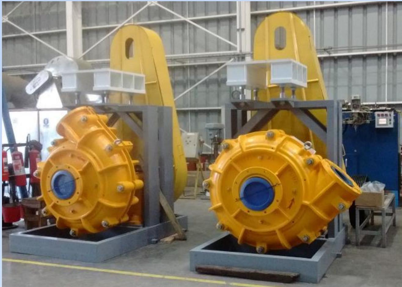
MA / MAR – Bomba Centrífuga Horizontal Heavy Duty
