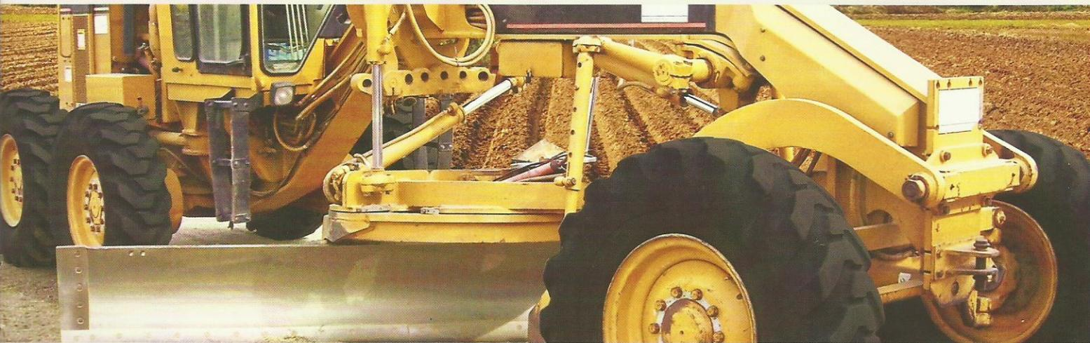
METISA manufactures tractor parts capable of reducing the physical strain and increasing the productivity, both in the field and in the cities. These are track shoes, grouser bars, graders blades, cutting edges, end bits, hot cupped end bits, teeth, shanks, tips and adapters, all of them made of either high-carbon steel or micro-alloyed steels with proper heat treatment for more resistance and durability.
