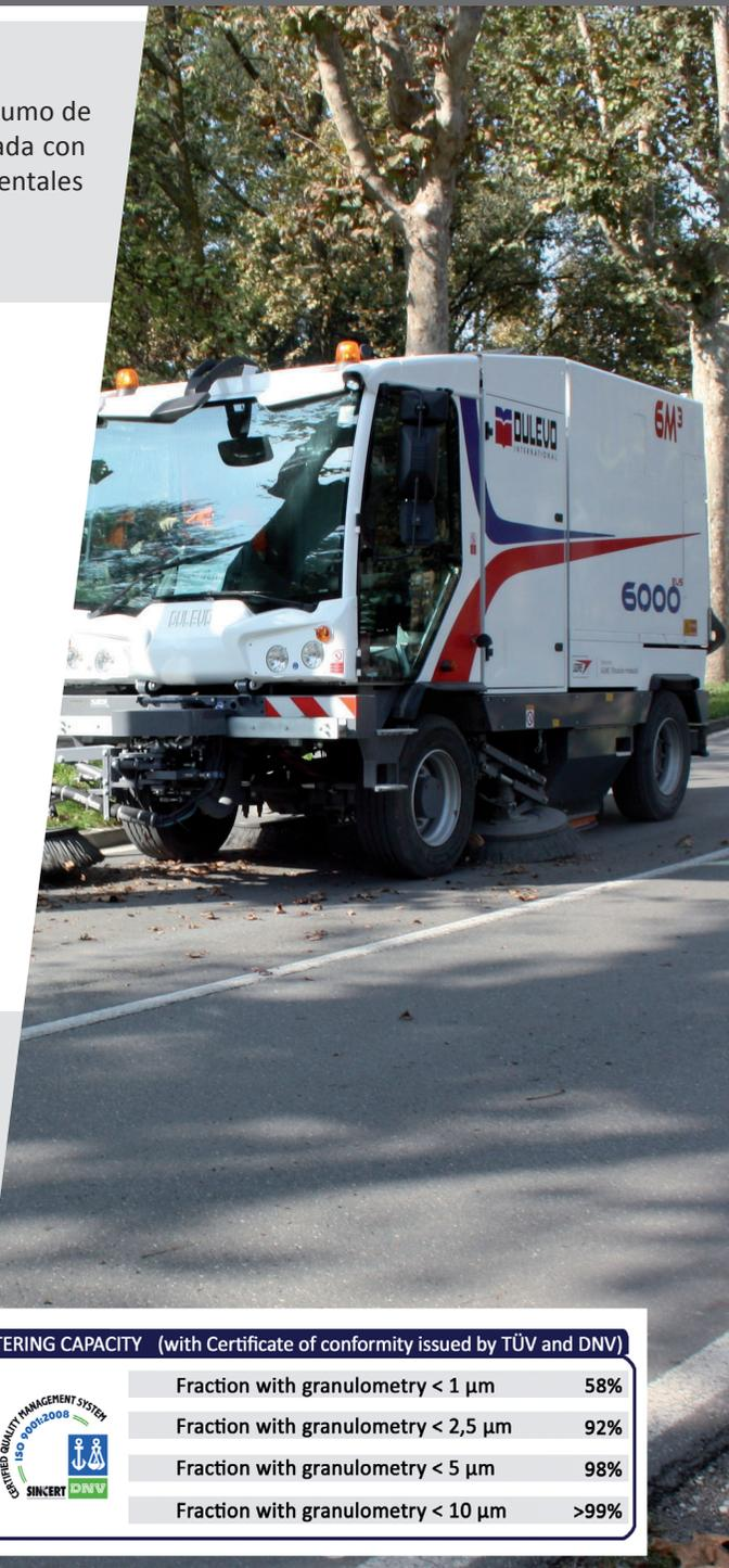
**FILTERING CAPACITY** (with Certificate of conformity issued by TÜV and DNV)
