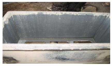
Wear inside concrete moulds
