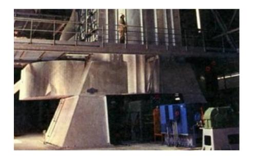
Chute under the table of the roller mill. HARDOX 400.
