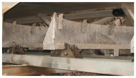
122 pieces of 10 mm HARDOX 450 replacing St52. Two years without any wear.
