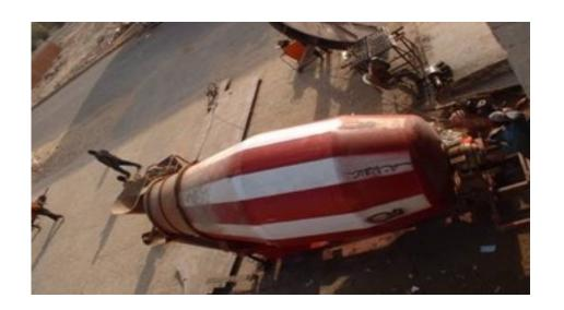
Extended body from size 4m3 TO 7m3, Made out of HARDOX 400. Internal mixing blades made out of HARDOX 400
