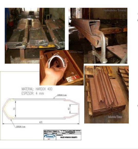
To produce moulds, that are putting after on the floor of the flats.
