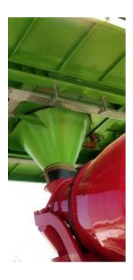
Drain chute to load the trucks. HARDOX 400
