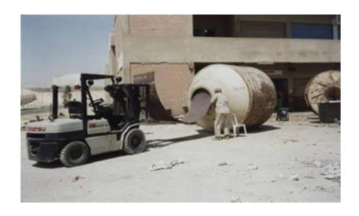
Jonson Mixer drum type Body and mixing paddles made out of HARDOX 400.
