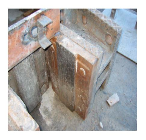
VERTICAL MILL for limestone/ marna HARDFACING plates (WEAR Resistant)
