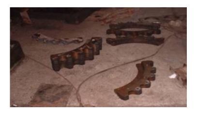
Clinker conveyor sprocket – Made out of HARDOX 500.
