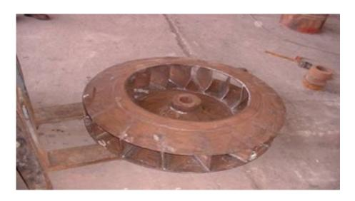
Deducting fan in steel mill made out of HARDOX 400
