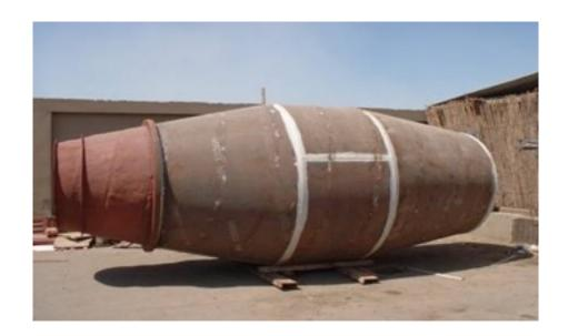
Complete body and mixing blades made out of HARDOX 400
