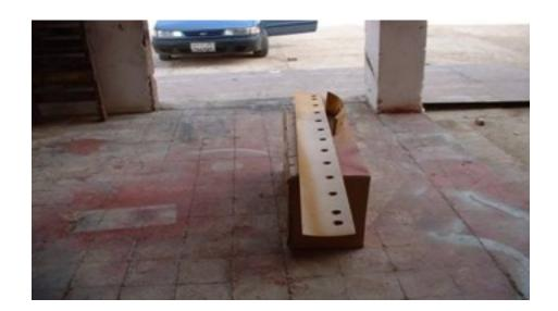
Cutting edge for grader made out of HARDOX 500.
