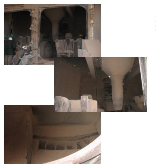
HARDOX 500 to HARDOX 600 using 8, 10, 15 and 20 mm.
