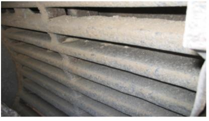
Linears out of HARDOX 500, 30 or 50 mm. In separators AWJ 30 mm HARDOX 500.
