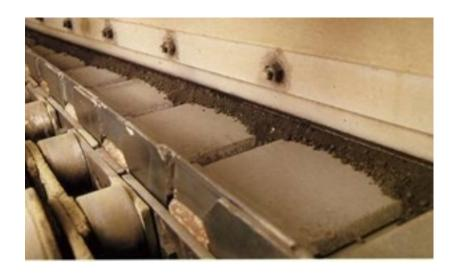
Other type of chain conveyor or Screw conveyor HARDOX 400
