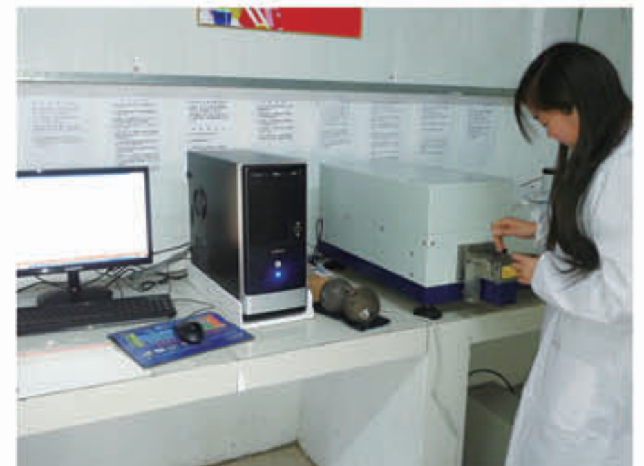
光谱仪用于检测化学成份 Spectrometer Is Used To Detect Chemical Composition
