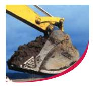
Designed for excavating in moderate to heavy abrasion applications such as shot rock, stratified material, and other abrasive conditions.
