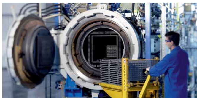
Element Six state-of-the-art sinter hip furnaces enable us to produce high quality tungsten carbide inserts to meet our customers' specific requirements.
