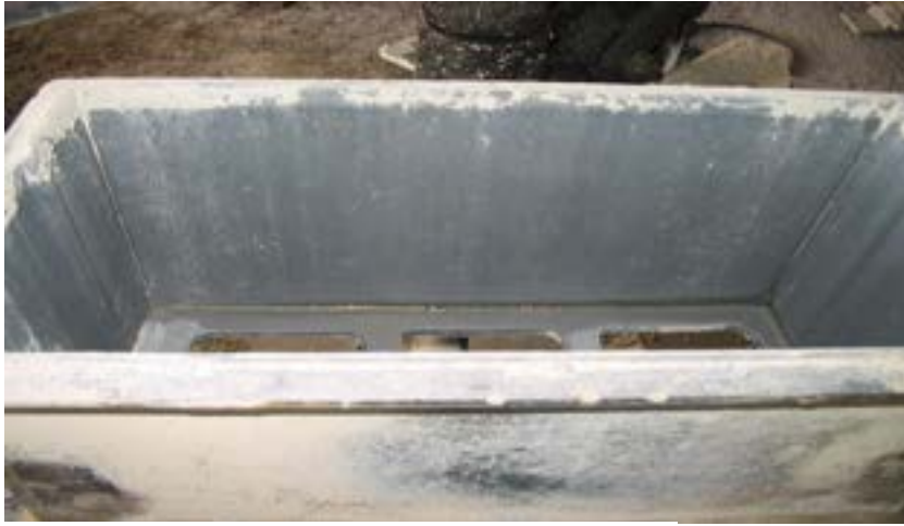
Wear inside concrete moulds
